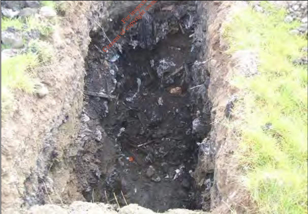
Photograph No.4 Waste material encountered in TP-9
