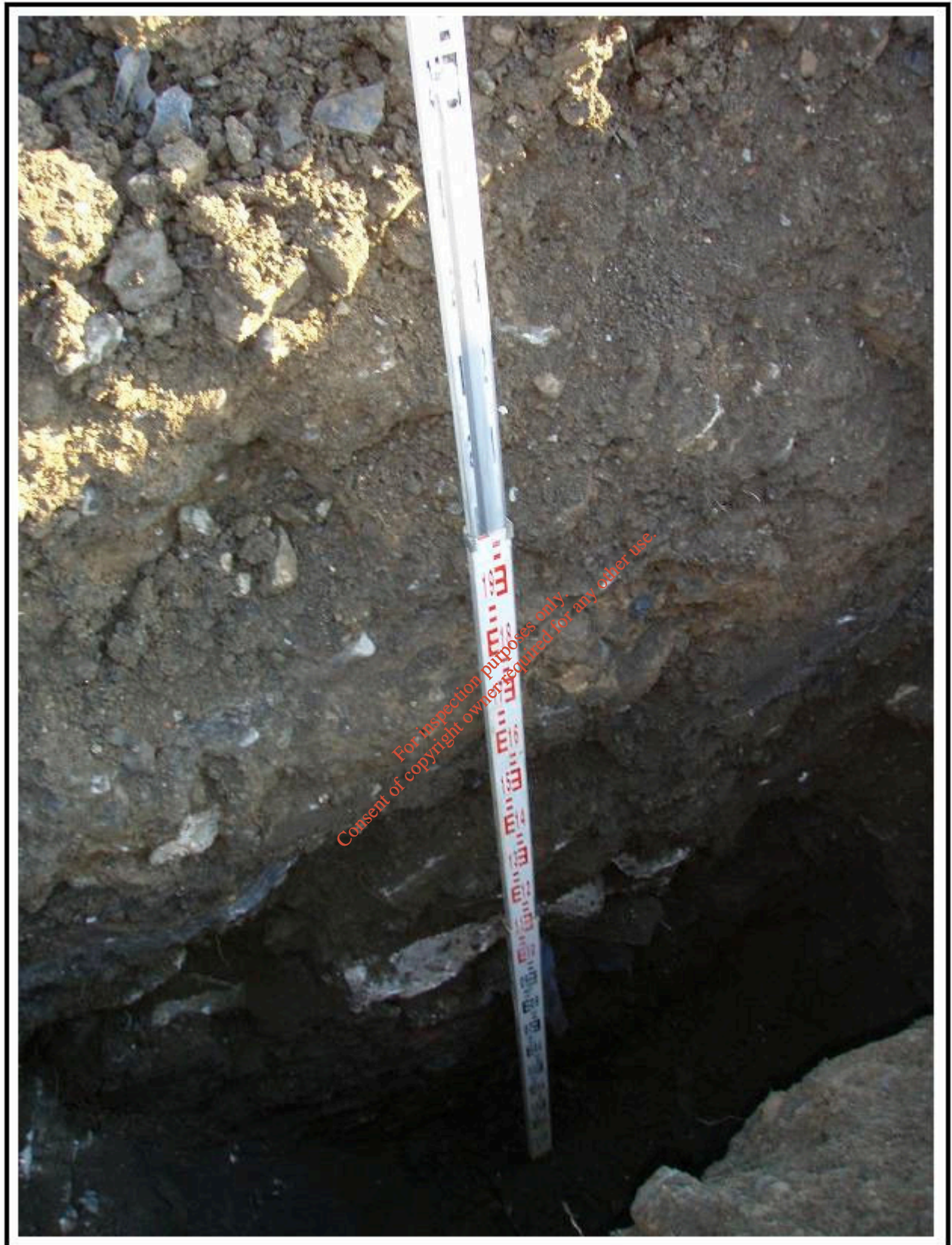
Plate A11: Profile of overconsolidated subsoil with alternating layers of very soft to stiff material in trial hole no. 11. Here some buried pieces of concrete are seen at depth. No topsoil has been emplaced above this material as of yet, and the ground is bare.
