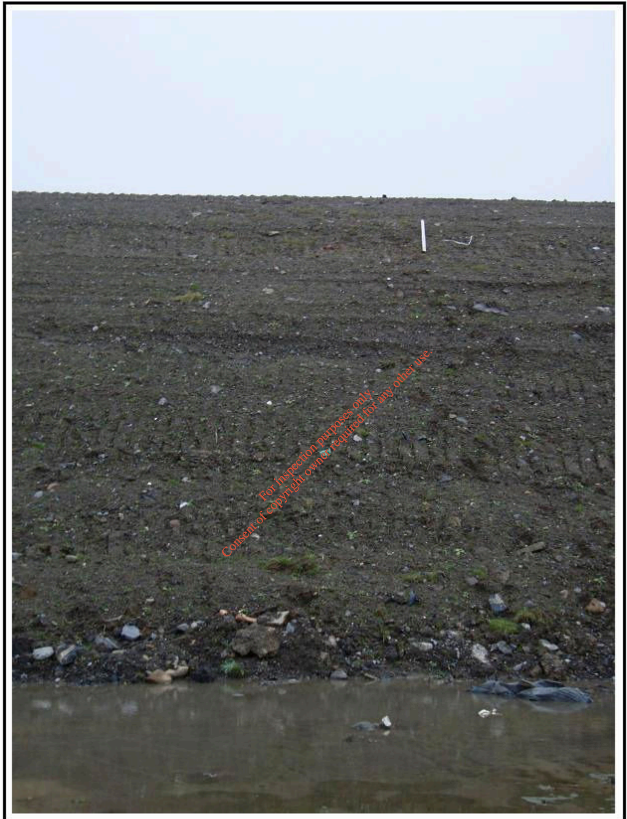
Plate A15: Profile of relatively shallow, recently-lain topsoil overlying overconsolidated subsoil at the northern side of the main eastern fill area. This material is very clean also.
