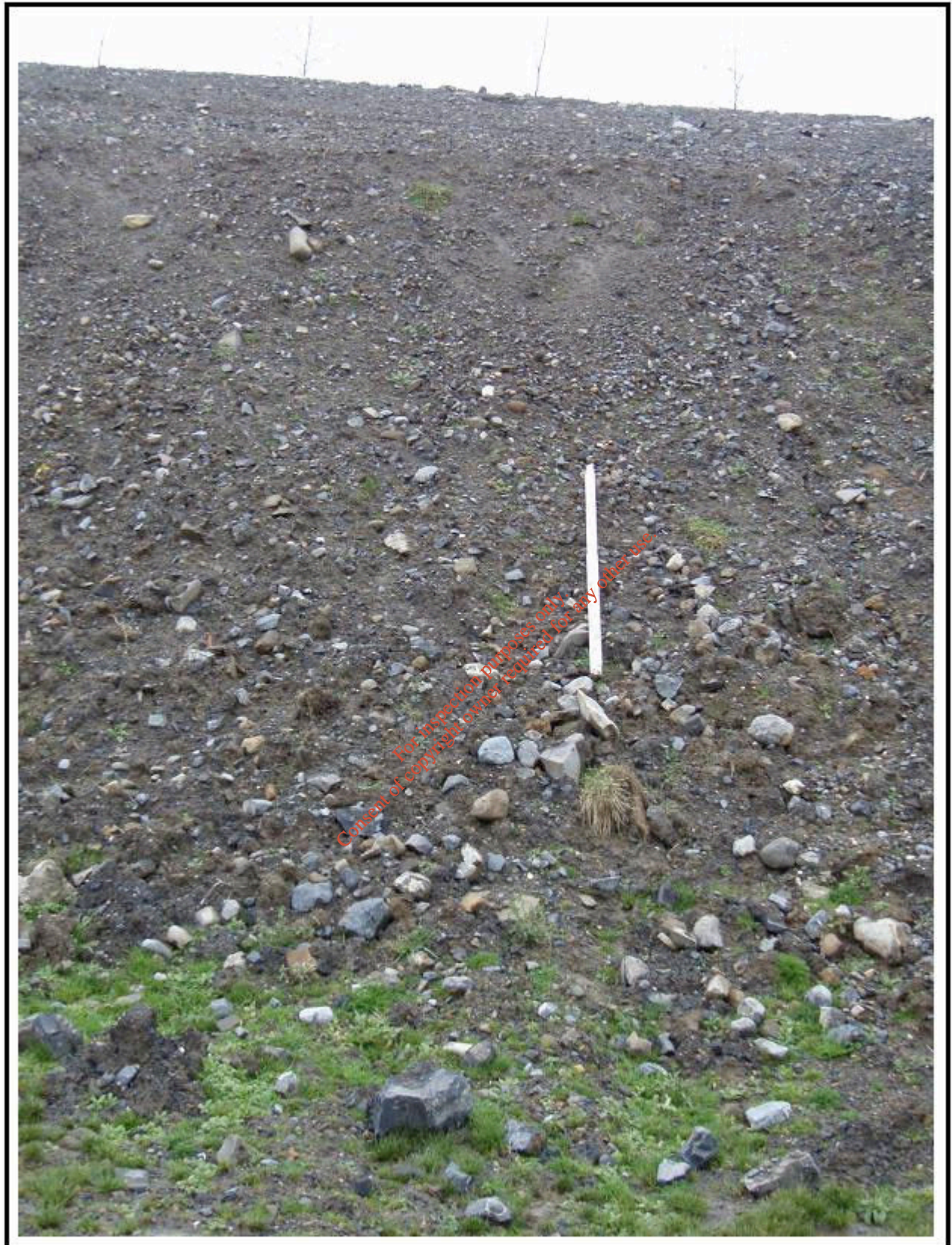
Plate A18: Profile of exposure into subsoil at the northwestern extreme of the main pit area. This material is clean, and again gets more gravelly and 'bouldery' at the base.
