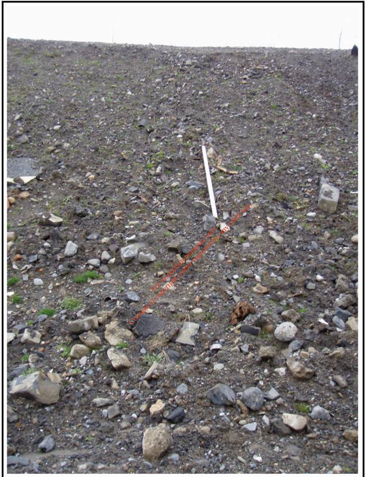
Plate A17: Profile of exposure into subsoil at the northeastern extreme of the main pit area. This material is clean, and gets more gravelly and 'bouldery' at the base.
