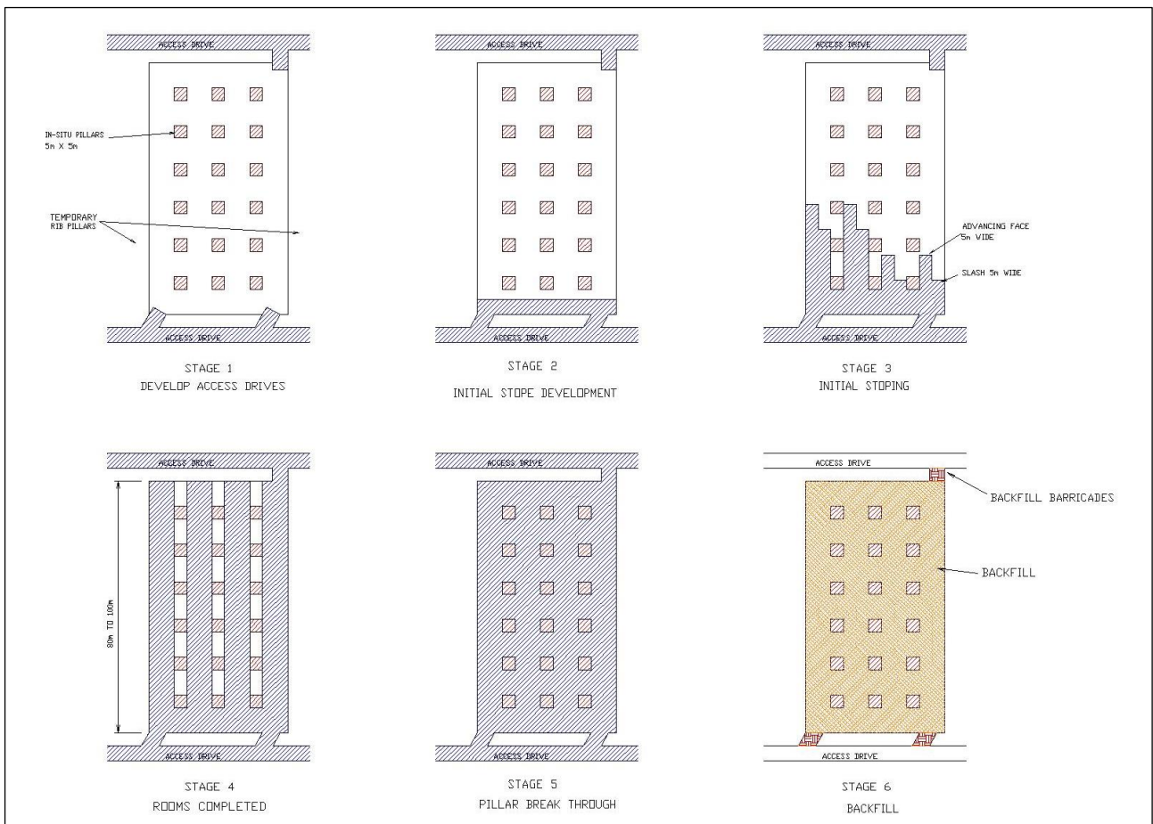
Figure 2.6: Room and pillar mining method
