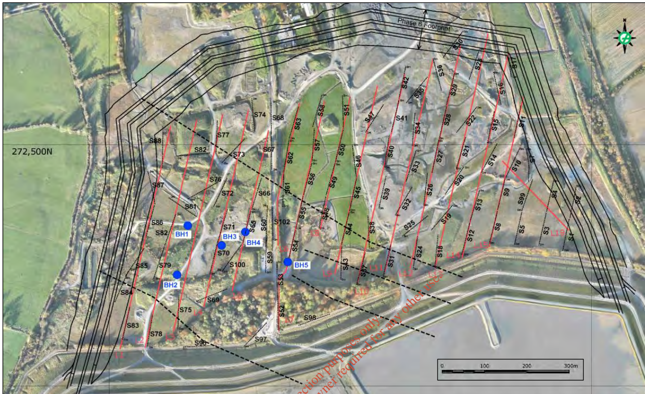
Figure 4: Location of Boreholes (plotted over recent aerial photograph of the Stage 6 TMF footprint)
