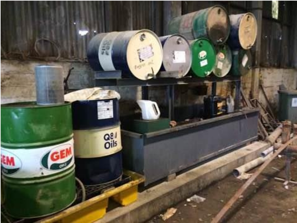
Figure 2 Garage oil bund
