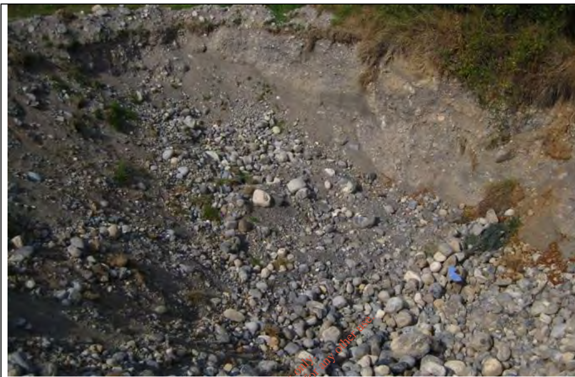
Photograph No: 3 Example of natural gravel sequence beneath site.
