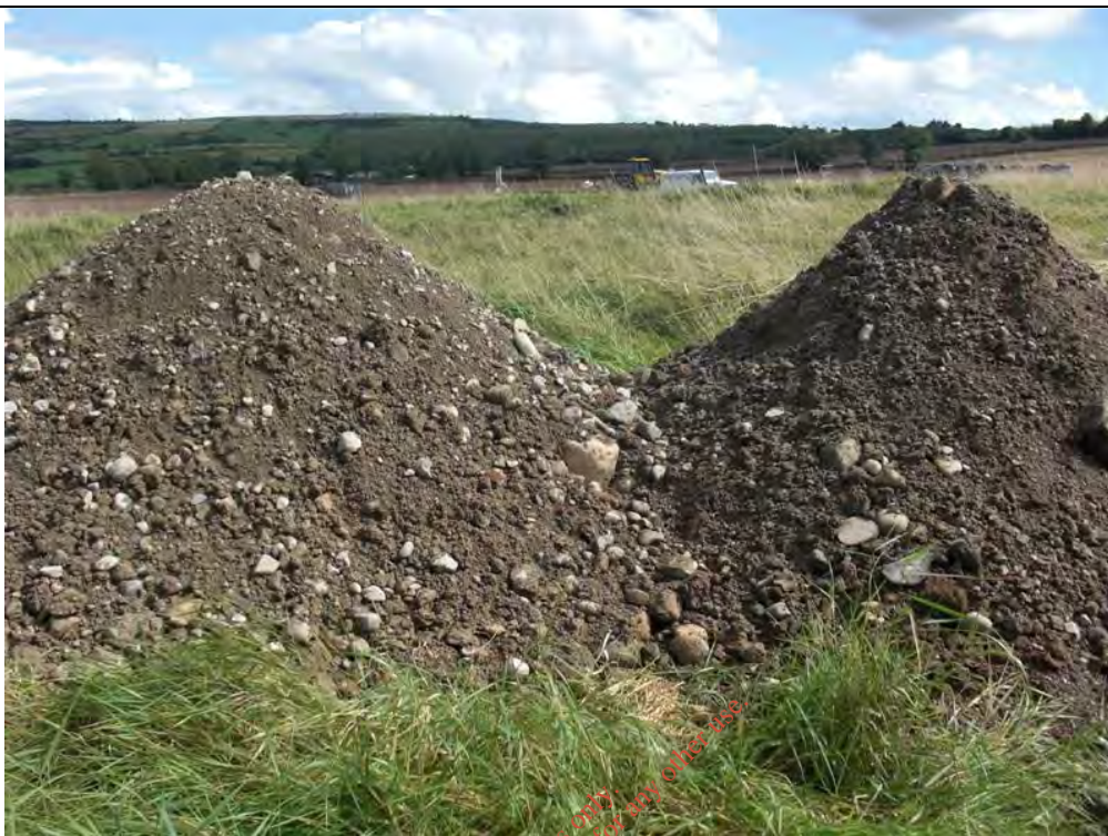
Photograph No: 5 Material used to cap waste body at location TP04.
