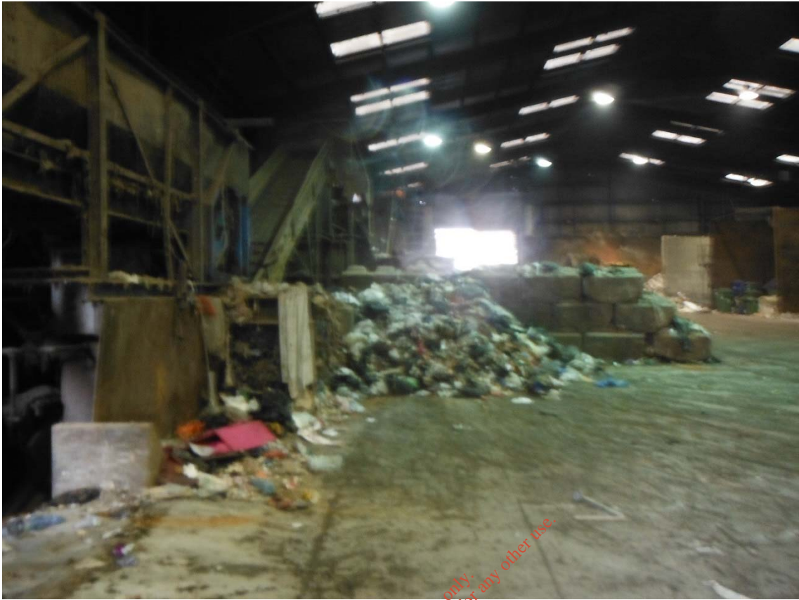
Figure 1.17: MRF: MMW Tipping Area, Bag Opener & Conveyor
