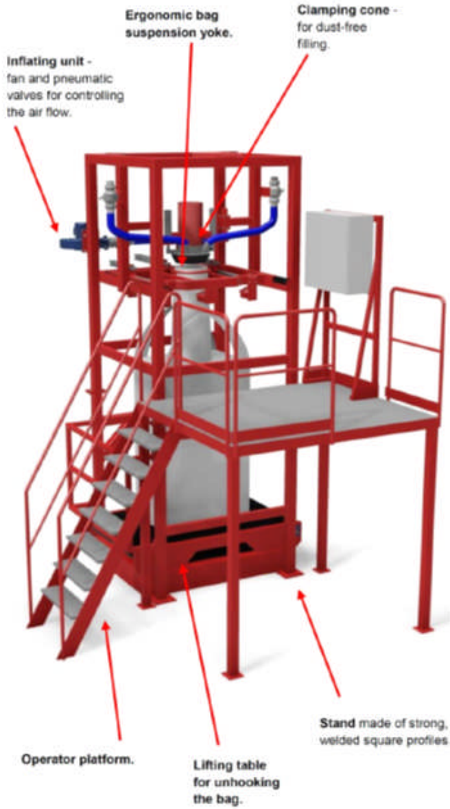
Figure 4: Details of components of bagging system
