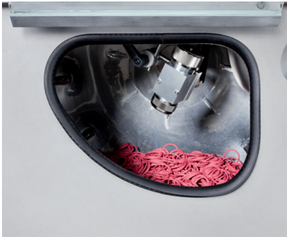
View of the inside of the drum with coated O-rings
