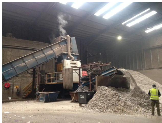
Discharge from solid recovered fuel production facility (Untha 1) in Building 2
