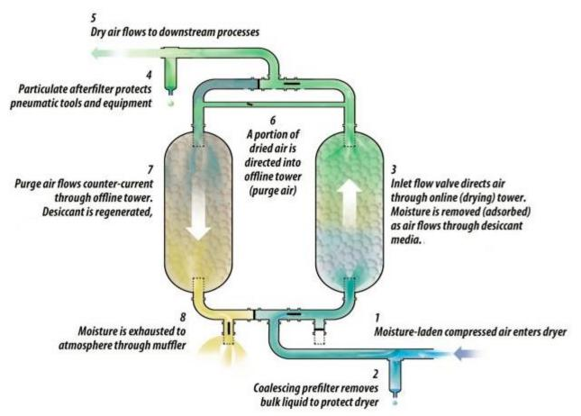
Each of the dryer's onsite have the capacity to dry 28.2 m3/min of compressed air. The spec sheet also notes that the nominal purge rate for the regenerating tower is 15% of total capacity, or 4.23 m3/min. However, the demand for instrument air at the time of audit was only 3m3/min which indicates the towers
