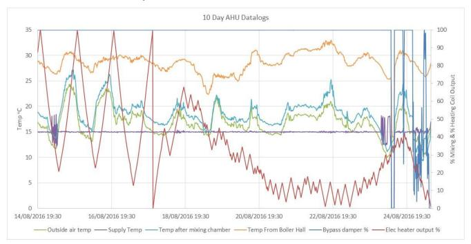
From the above graph it can be seen that the supply temperature is in general controlled to very tight limits as can be seen by the flat line. Where there are deviations in this temperature (such as on the 15<sup>th</sup> of August) the heating coil output tends to react very slowly, but over a wide range. This suggests that the control response time needs to be altered.
