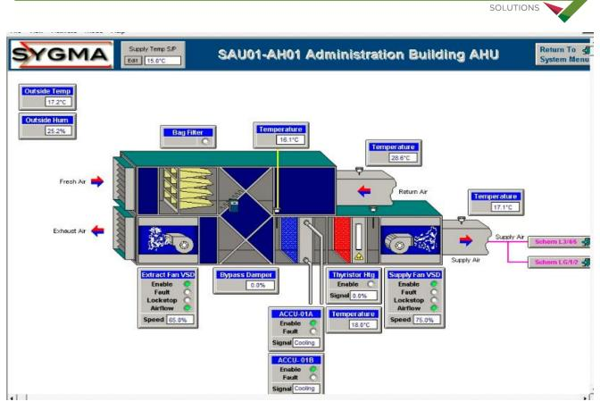
During the audit a number of datalogs which were available on the BMS were downloaded and subsequently plotted against each other to examine how the AHU was controlling. The default amount of data stored on the BMS is 10 days.
