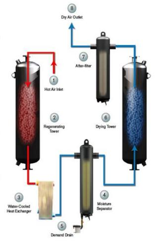
This system would require some pipework reconfiguration so that the refrigerated dryer is bypassed allowing hot compressed air to be sent to the desiccant dryer and a water cooled heat exchanger would be required. However, the annual savings from this measure would be 232,600 kWh, or €19,700.
