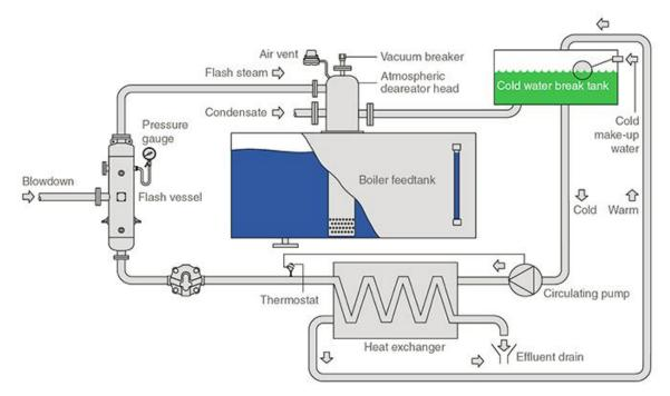
As the blowdown is periodic it is necessary to install a break tank with a circulating pump which is operated on a thermostat to take the heat when it becomes available.
