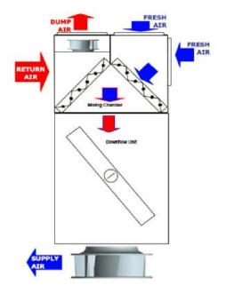
Due to the moderate climate in Ireland, free cooling is possible for a high % of the year. Based on 2014 weather data, the number of hours the weather was below 16 °C was 7,030 hours, or 80% of the time. The potential electrical savings from installing a free cooling unit, and using the Mitsubishi units as standby units only, would be approximately 113,000 kWh, or €9,600.
