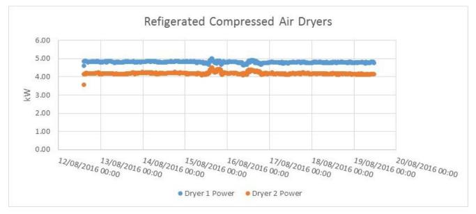
The results show that both dryers have a steady power consumption throughout the course of the week. There were small fluctuations on the 15<sup>th</sup> and 16<sup>th</sup> of August which corresponds to the fluctuations in the compressor power on those dates (see section 3.3.2).
