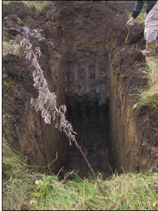
Plate 5: Section from Trial Pit 5 – note v thin layer of fill (c.0.3m)
