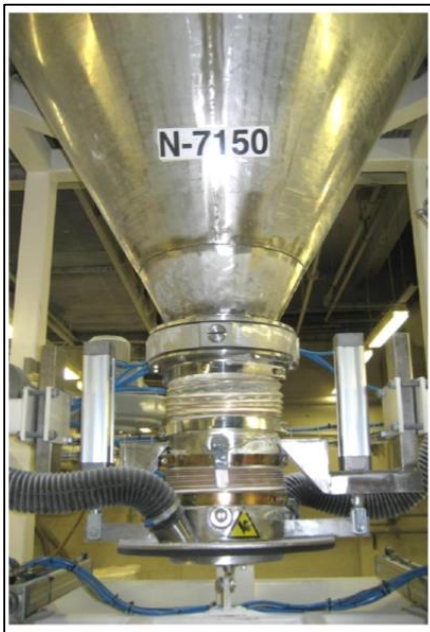
Figure 7: Close-up view of the clamping cone
