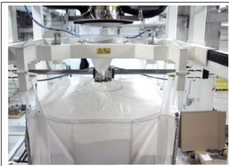
Figure 8: Automatic bag welder with welding in progress
