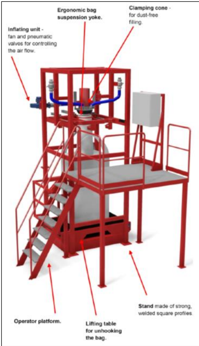
Figure 4: Details of components of bagging system
