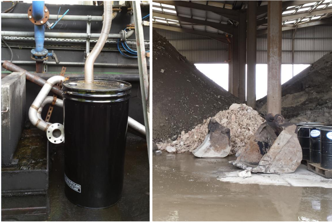
Figure 12 (a) Water trap for controlling fugitive emissions. The drum contains water plus a deodorising chemical. (b) Unenclosed, covered soil treatment area.
