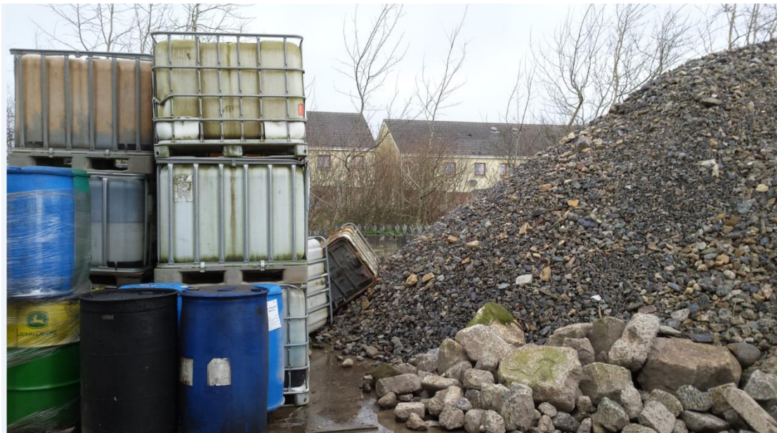
Figure 13 Recovered rubble and stone stored outdoors, in addition to empty drums and other containers. The stone and rubble are screened out of waste soil accepted at the installation for treatment.
