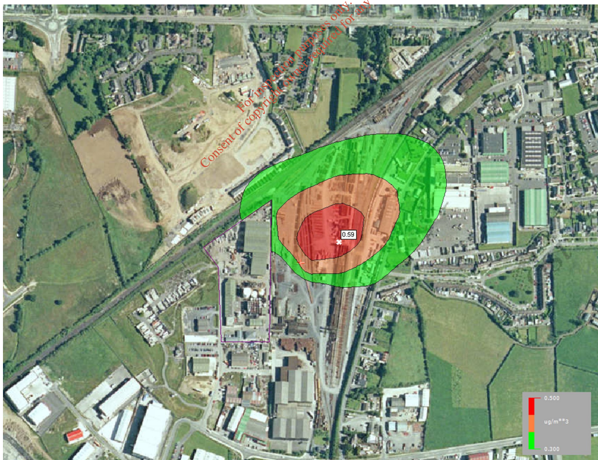
Figure 14.2: Results of VOC Modelling from the RTO (annual averages but excludes background)
