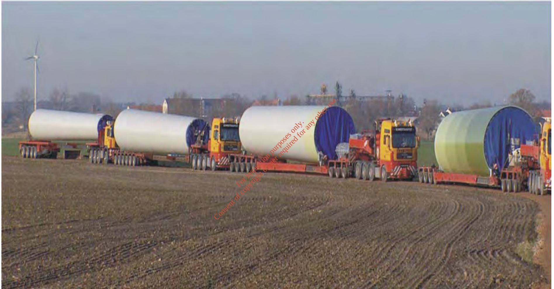
Figure 13.1: Typical Delivery of Wind Turbine Tower Components
