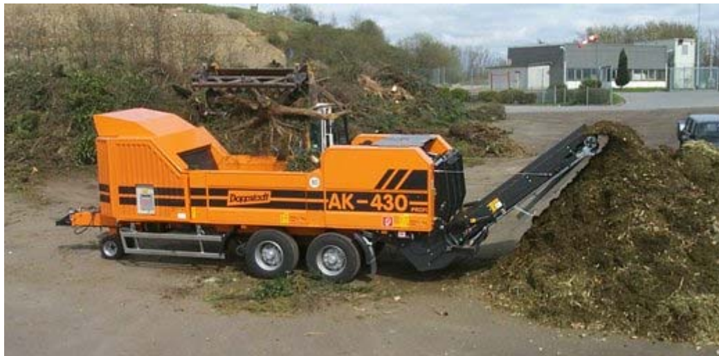
Photo D.2 1: Typical Shredding unit ( www.doppstadt.com )
