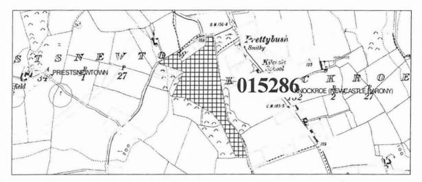
This proposal specifically relates to the filling of a low lying area of the site with up to  $150,000m^3$  of excavated material arising from the works on the proposed Southern Access Road / Drummin Link. The area to be filled is the valley / depression, along the western side of the site. It is proposed to bring this depression to the same level as the adjoining lands.
