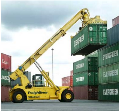
Plate 3.8 Typical Reach Stacker
