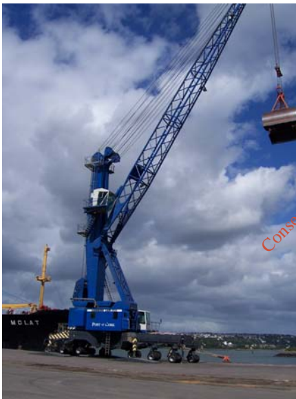
Plate 3.9 Typical Harbour Mobile Crane
