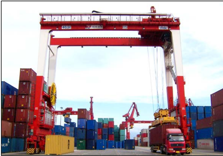
Plate 3.6 Typical RTG Yard Crane
