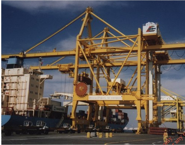
Plate 3.4 Typical Rail Mounted Ship to Shore Crane
