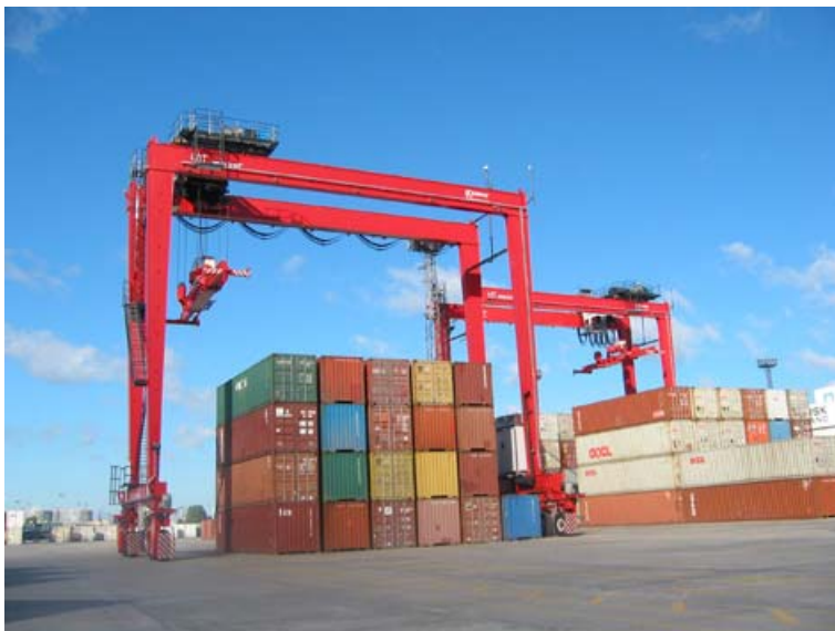
Plate 3.5 Typical RTG Yard Crane
