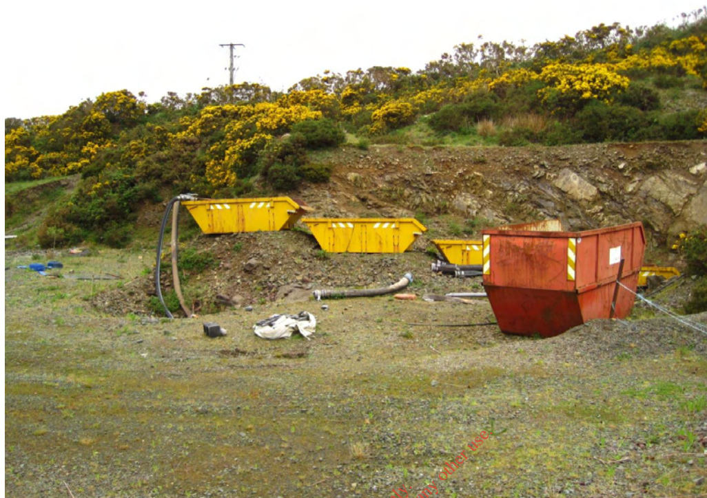
Plate 6-3 Former Settlement Tank System (now disbanded)
