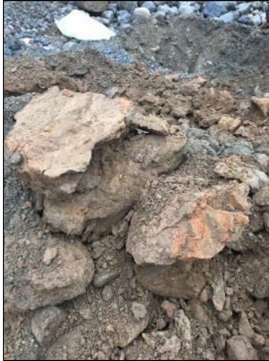
Figure K: Hard laminated clay and lacustrine deposits from TP15-12
