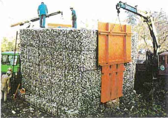
■ Two full size gabion walls under test programme in Italy.
