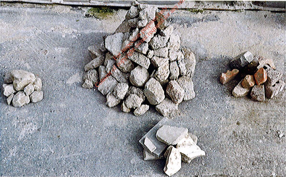
Photo No.6 shows sample separated into aggregate, concrete, ceramic and brick.
