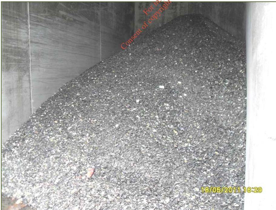
Photograph D.2.3: Clean/separated glass cullet output
