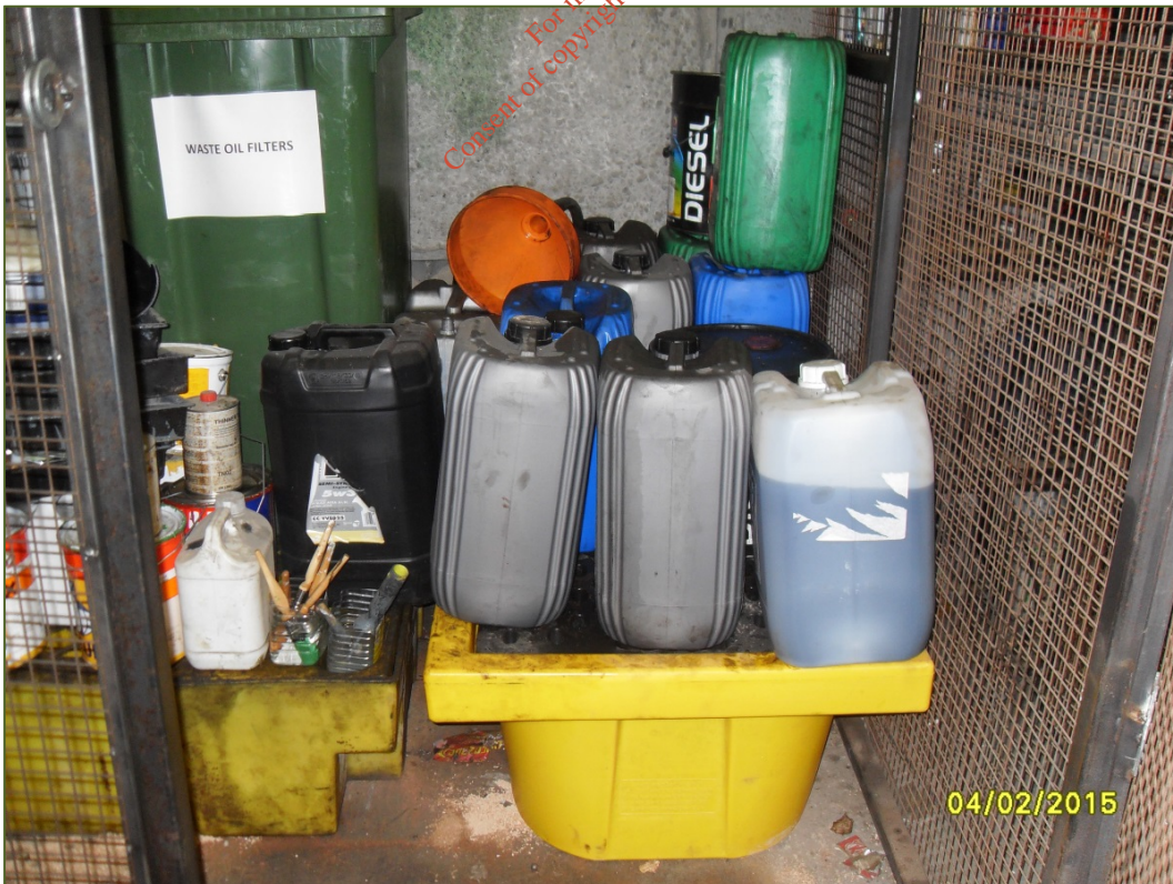
Photograph D.1.14: Spill pallet in garage building
