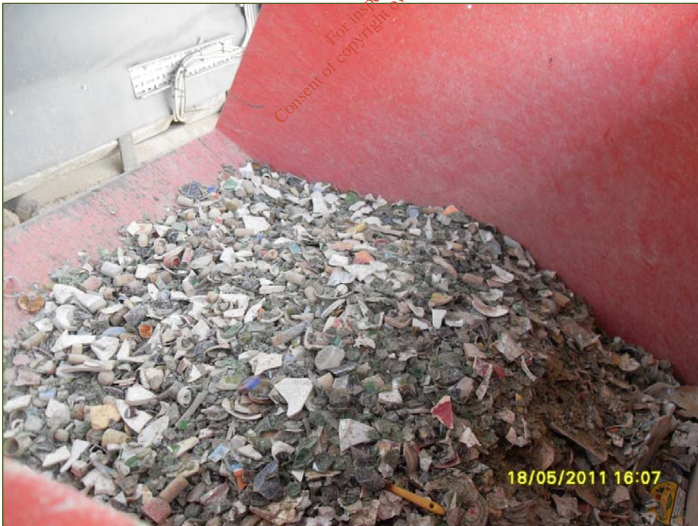
Photograph D.2.11: Residual waste from the Drying Plant
