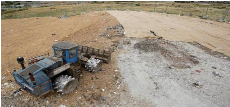
Figure 2.5: Typical landfilling operation using waste compactor
