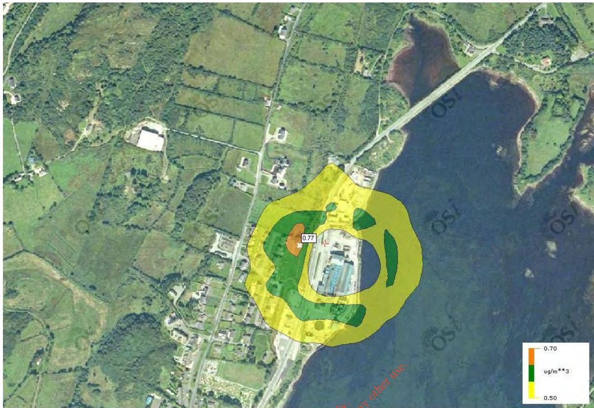
Figure 3.10: Scenario B Maximum 1-hour Hydrogen Sulphide Concentrations (Contours represent 0.7\mu\text{g}/\text{m}^3 , 0.6\mu\text{g}/\text{m}^3 and 0.5\mu\text{g}/\text{m}^3 ). Short Term EAL for the protection of human health 150\mu\text{g}/\text{m}^3 .
