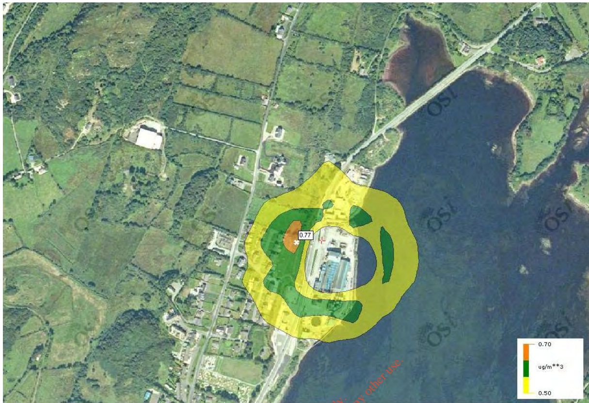
Figure 3.11: Scenario B Maximum 1-hour Mercaptan Concentrations (Contours represent 0.7\mu\text{g}/\text{m}^3 , 0.6\mu\text{g}/\text{m}^3 and 0.5\mu\text{g}/\text{m}^3 ). Short Term EAL for the protection of human health 300\mu\text{g}/\text{m}^3 (as methyl mercaptan).
