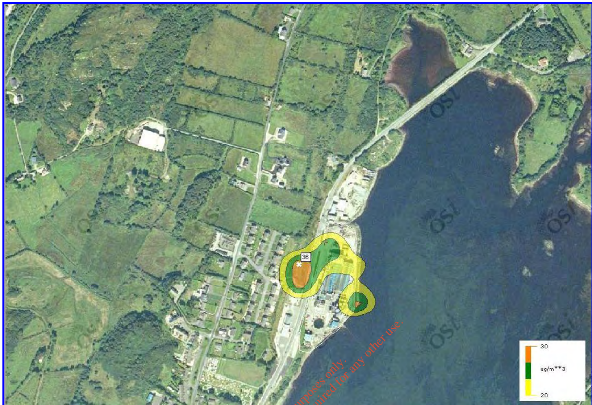
Figure 3.8: Scenario B Maximum 1-hour Ammonia Concentrations (Contours represent 30\mu\text{g}/\text{m}^3 , 25\mu\text{g}/\text{m}^3 and 20\mu\text{g}/\text{m}^3 ). Short Term EAL for the protection of human health 2500\mu\text{g}/\text{m}^3 .
