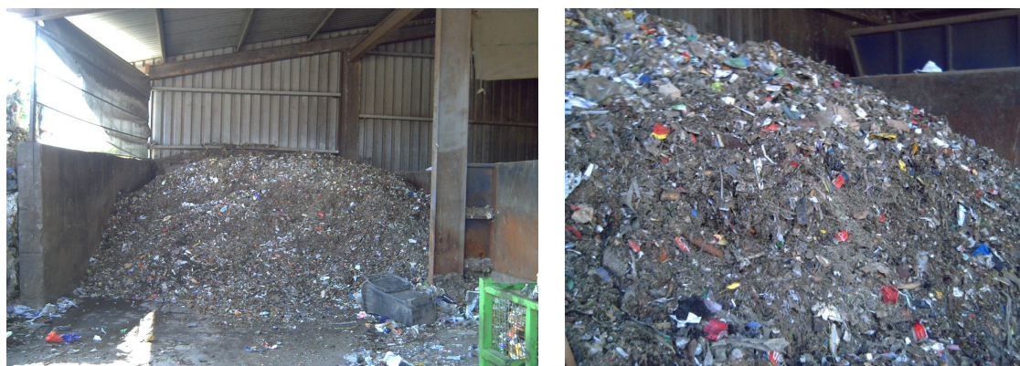
Figure 1 Typical MBT fines produced from black bin municipal waste
