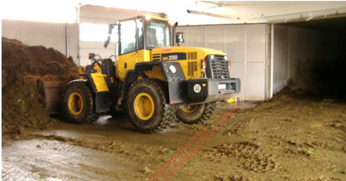
Figure 5 Filling of a fermentation chamber with Bio-waste
