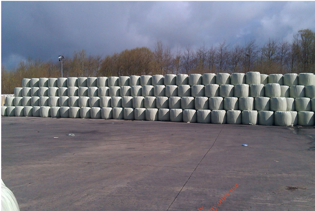
Photo 5 – External Storage of RDF Bales
