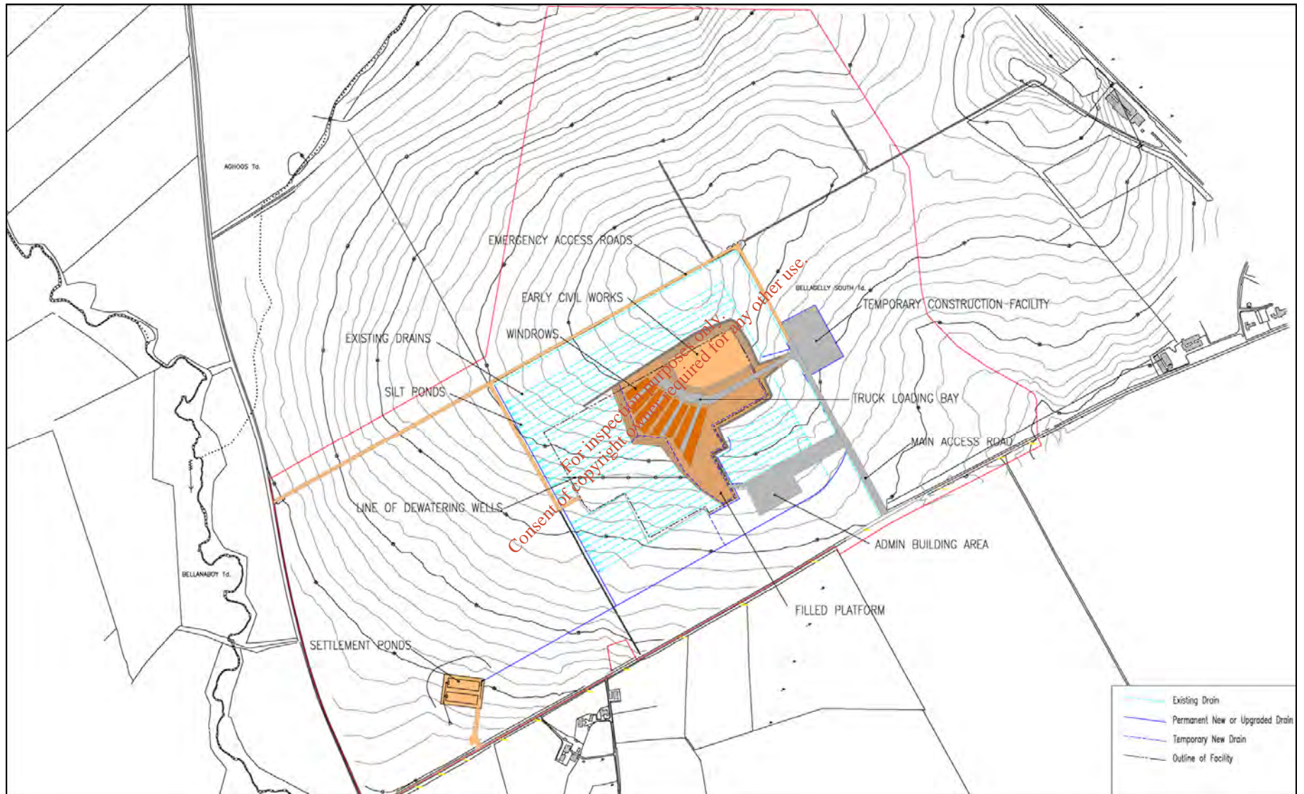
Figure 3.5 Peat Removal Intermediate Stage
