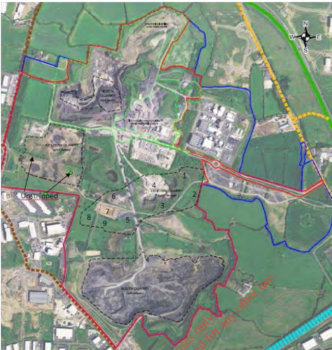
Plate 11.1 Aerial Photography of the Huntstown Quarry showing the four quarry areas and indicating the unquarried areas in the Central Quarry 1-9 and the unquarried areas in the Western quarry with arrow.
