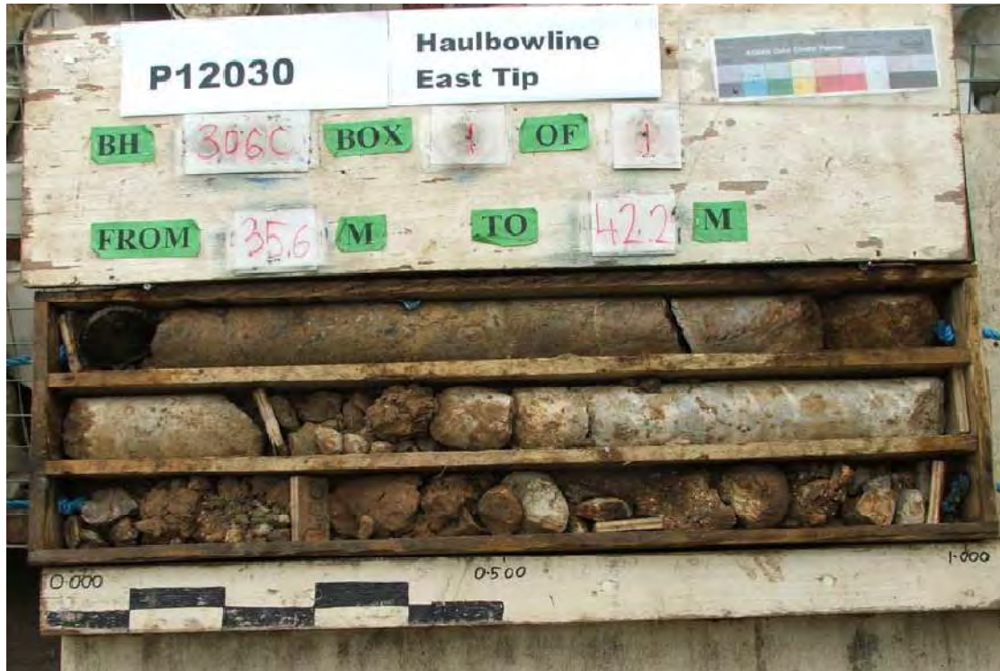
Photograph 13.4: Bedrock Core from BH306C – Significant Karst Solution of Limestone with Sand, Gravel and Clay Infilling
