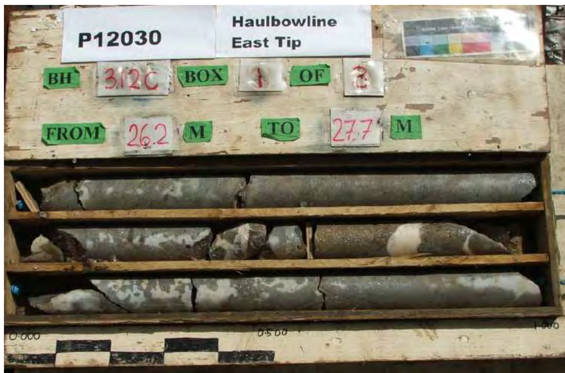
Photograph 13.1: Bedrock Core from BH312C – Competent Hard Limestone with Minor Solution Weathering Along Fractures
