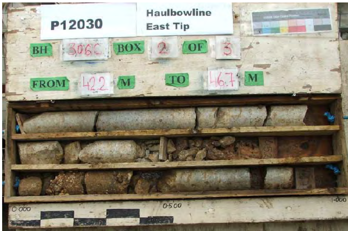
Photograph 13.5: Bedrock Core from BH306C – Significant Karst Solution of Limestone with Sand, Gravel and Clay Infilling
