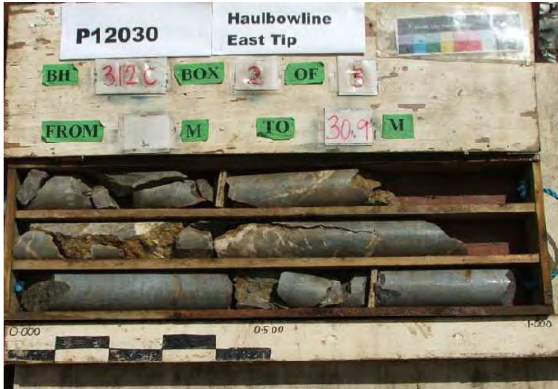
Photograph 13.2: Bedrock Core from BH312C – Competent Hard Limestone with Minor Solution Weathering Along Fractures
