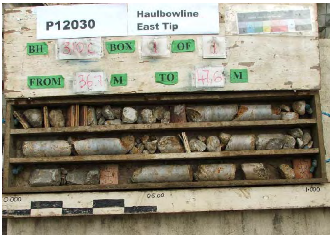
Photograph 13.3: Bedrock Core from BH310C – Karstified Limestone with Poor Core Recovery
