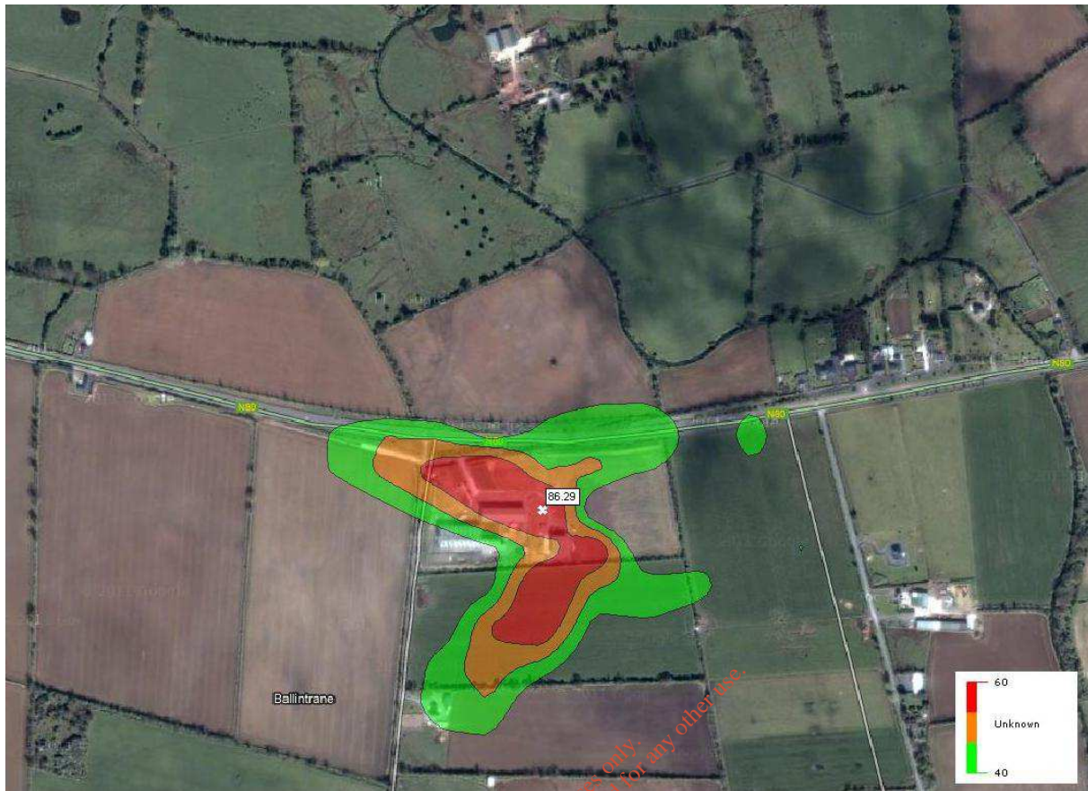
Figure 3.2: Scenario 4, 1-hour NO 2 Concentrations (Contours represent 60µg/m 3 , 50µg/m 3 and 40µg/m 3 ). Backgrounds not included. Statutory limit for the protection of human health 200µg/m 3 (as NO 2 ).
