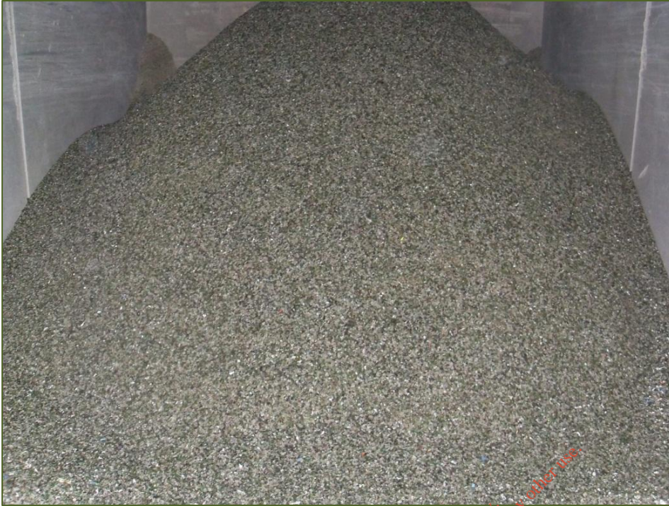
Photograph 2.21: Main Process output - Clean/separated glass cullet
