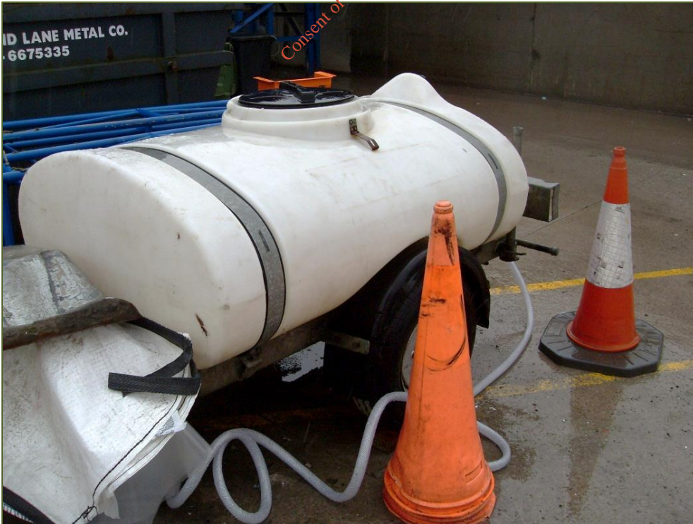
Photograph 2.48: Water bowser (for dust management)
