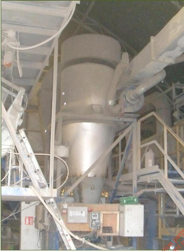
Photograph 2.33: Drying Plant - 'Cyclone' Dust Management System
