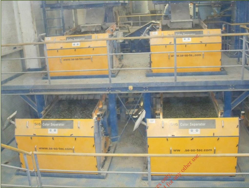
Photograph 2.13: Main Process Building – Spectrum Units (glass colour separators)
