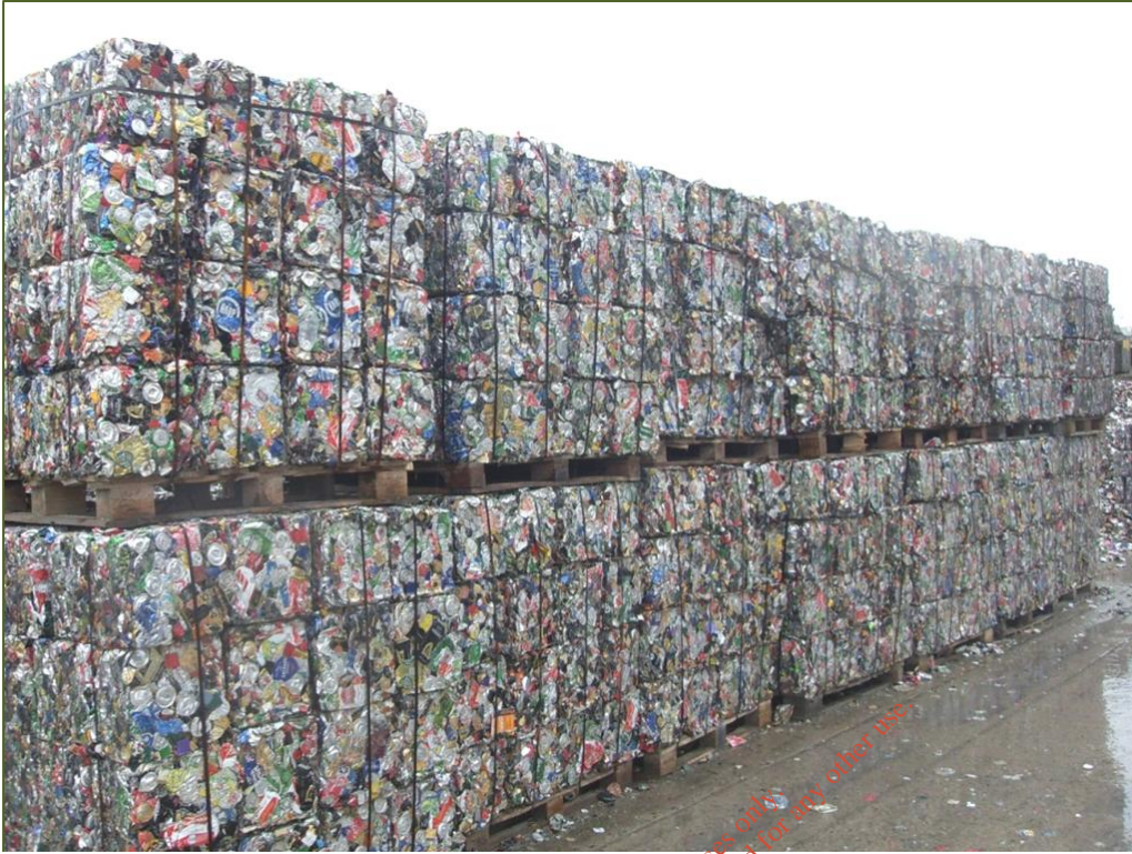
Photograph 2.19: Main Process output - Baled cans/metal storage
