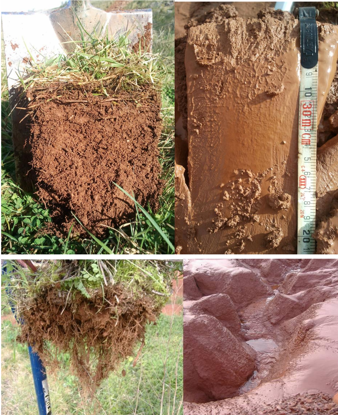
Plate 2. Examples of residue lacking of structure with increased erodibility risk in unamended residue (right) and formation of soil structure in restored residue (left)
