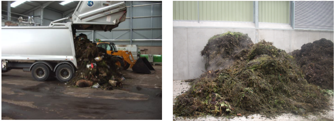
Fig. 4. Bio-waste being tipped at the Broadpath in-vessel composting facility in Devon (left) and material being held prior to processing (right).
