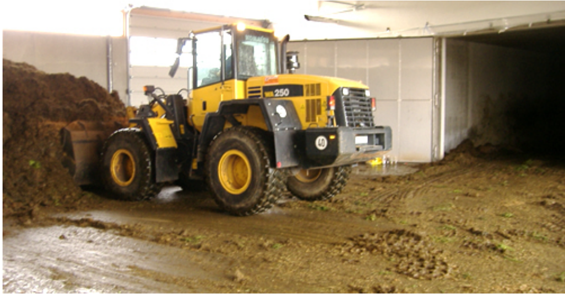
Fig. 7. Filling of a fermentation chamber with Bio-waste.
