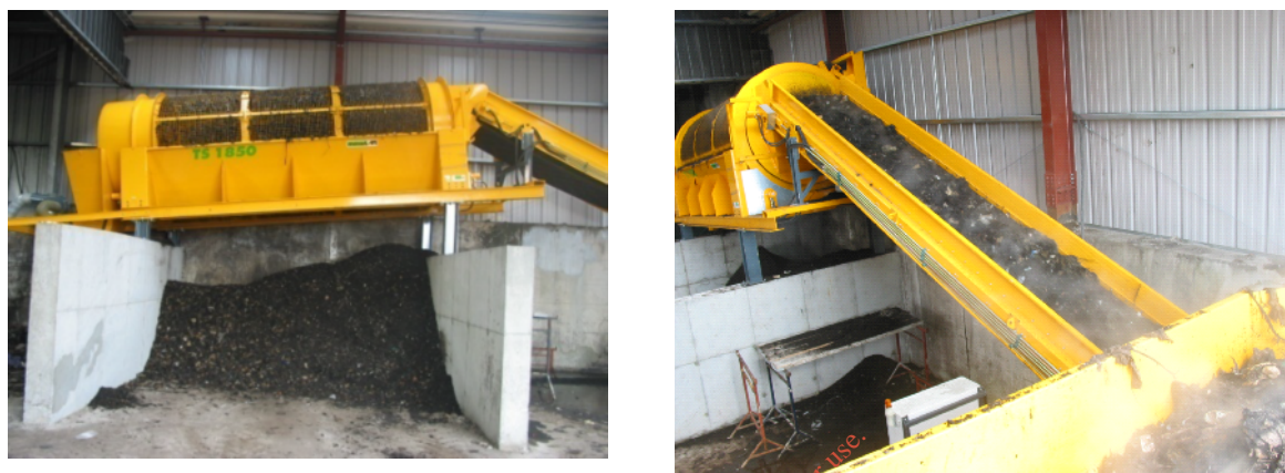
Fig. 17. Housed trommel screen illustrating multiple sections that produce different grades of compost and overs.
