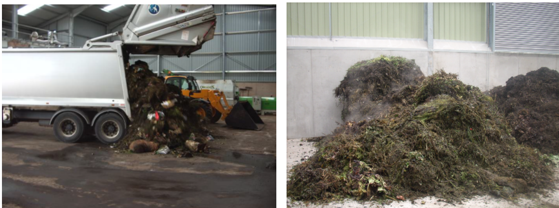
Fig. 5. Bio-waste being tipped at the Broadpath in-vessel composting facility in Devon (left) and material being held prior to processing (right).
