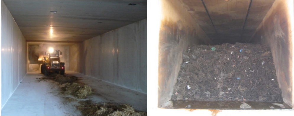
Fig. 9. Interior of fermenter prior to filling (left) and with bio-waste prior to fermenter sealing.
