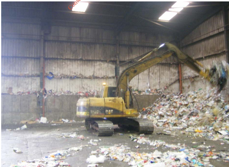
Figure 2.1: Dry recyclable reception area
