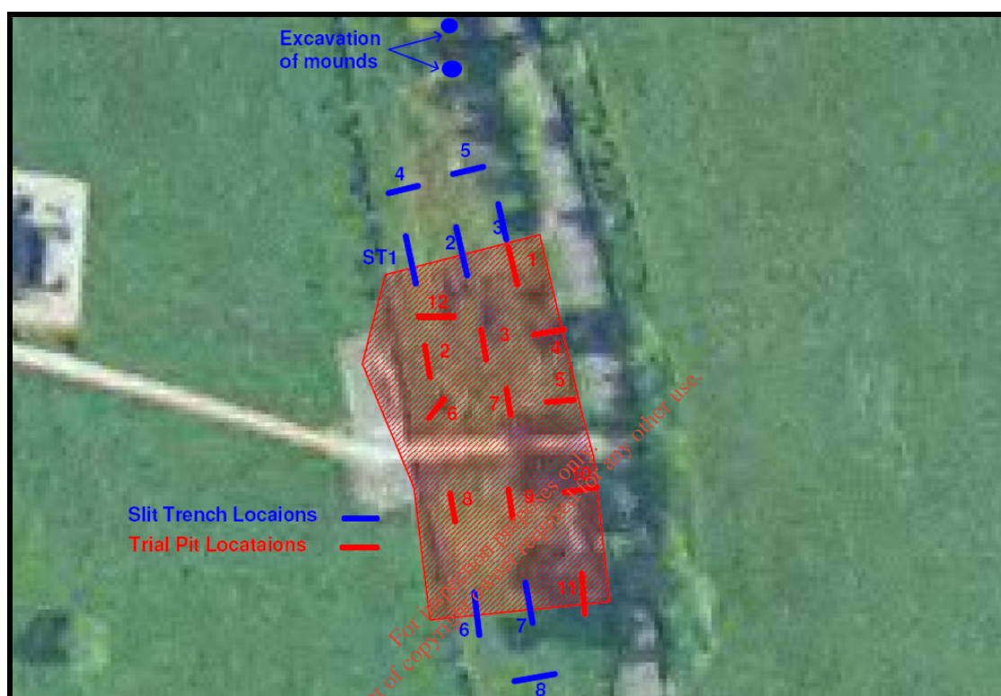
Fig. 3.3 - Slit Trench and Trial Pit Locations
