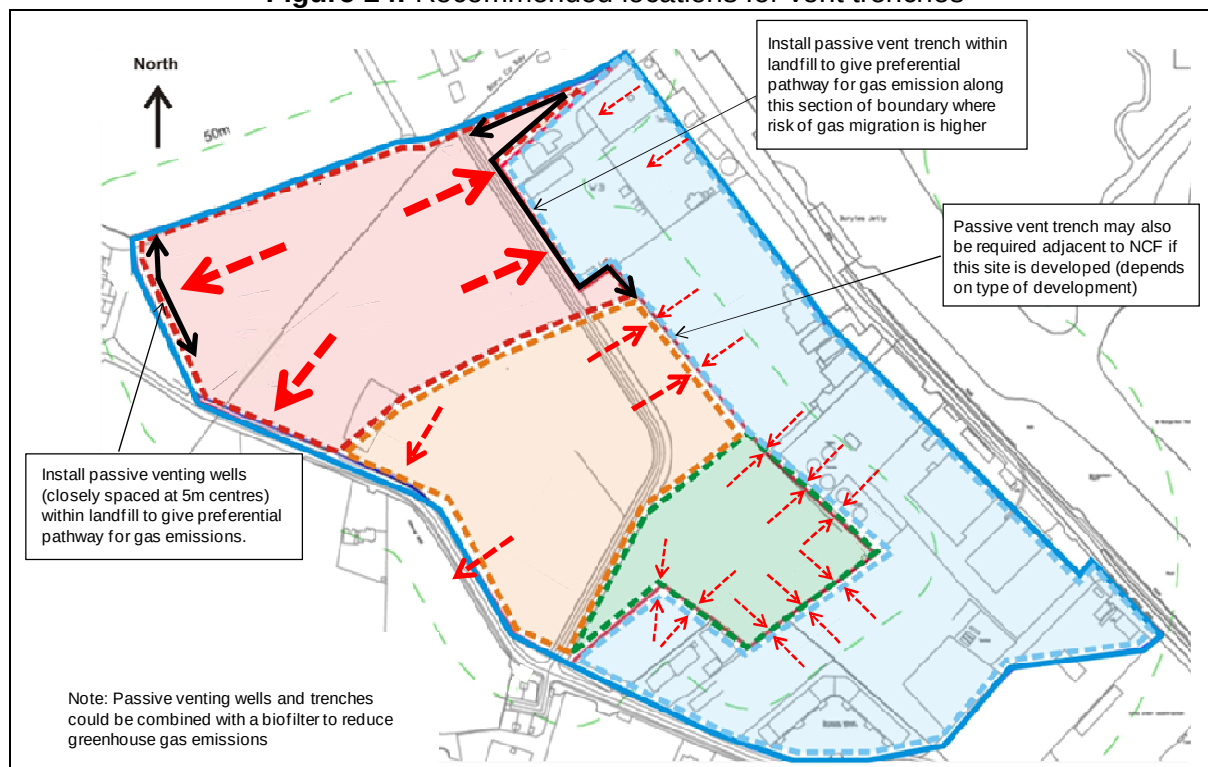
Figure 24: Recommended locations for vent trenches
