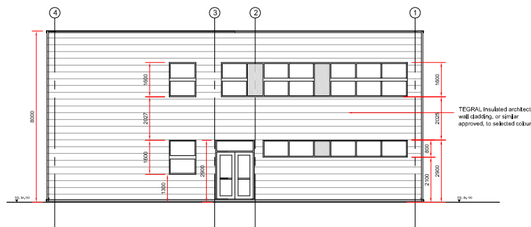
ADMIN/WELFARE BUILDING - WEST ELEVATION
