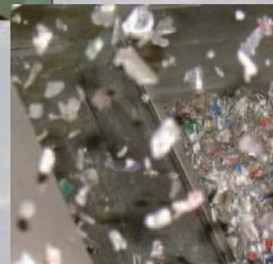
Aluminium dynamically ejected from metallics
