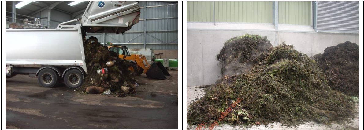
Figure 2 Bio-waste being tipped at the Broadpath in-vessel composting facility in Devon (left) and material being held prior to processing (right).
