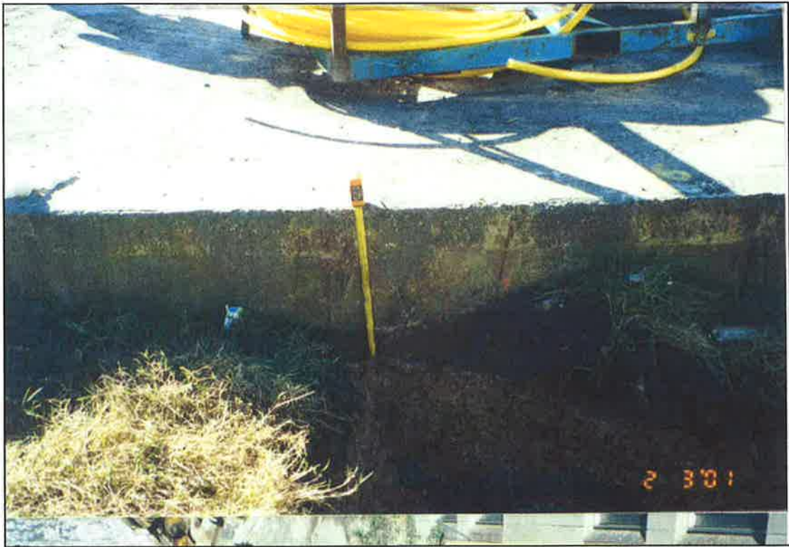
TP 36 View of 0.5m Thick Gas holder Base
