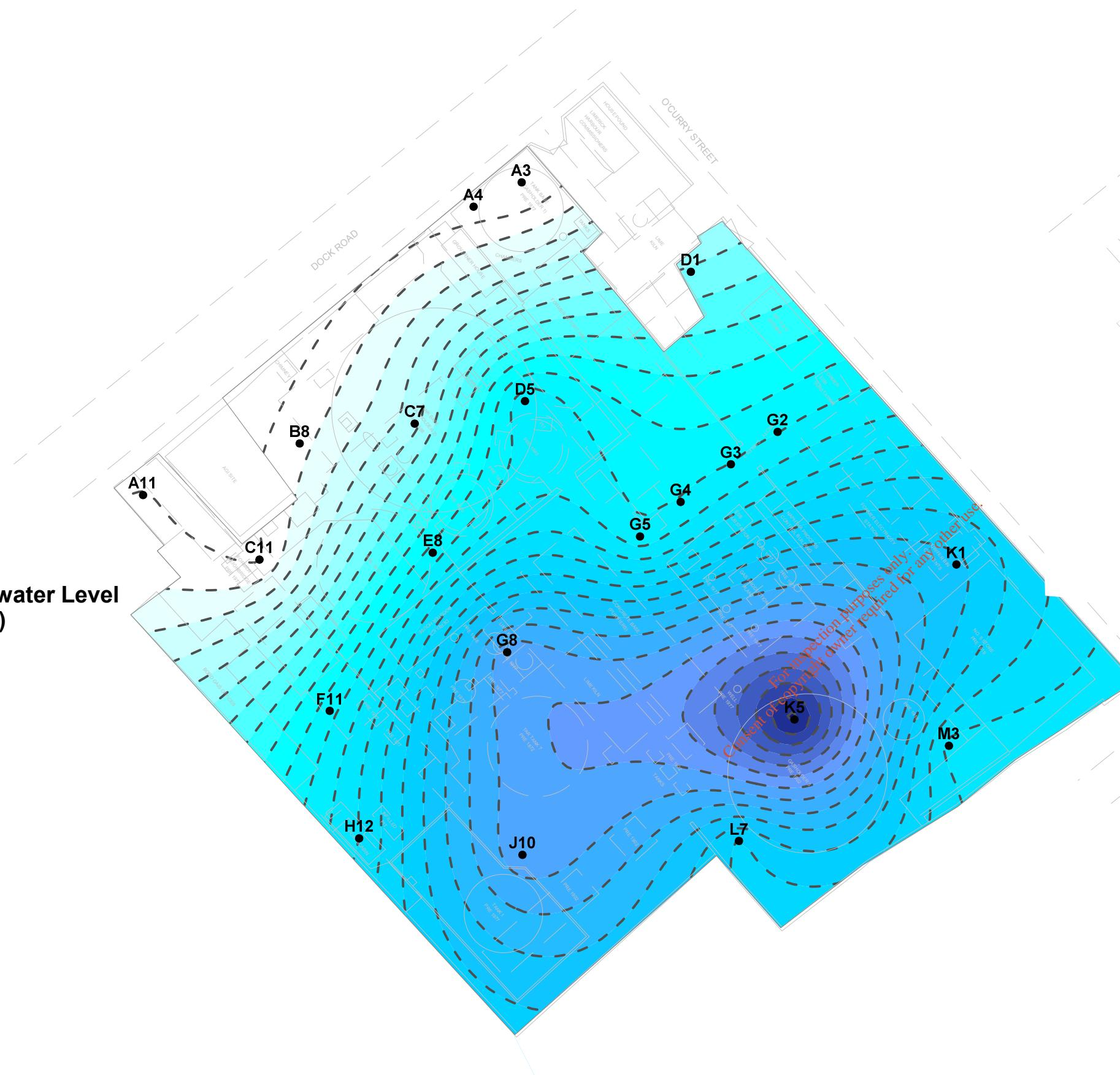
These plots have been produced using data obtained from the groundwater monitoring visit undertaken on 24-26/10/2011. Contours were plotted using the Kriging method based upon a 1m x 1m grid.
