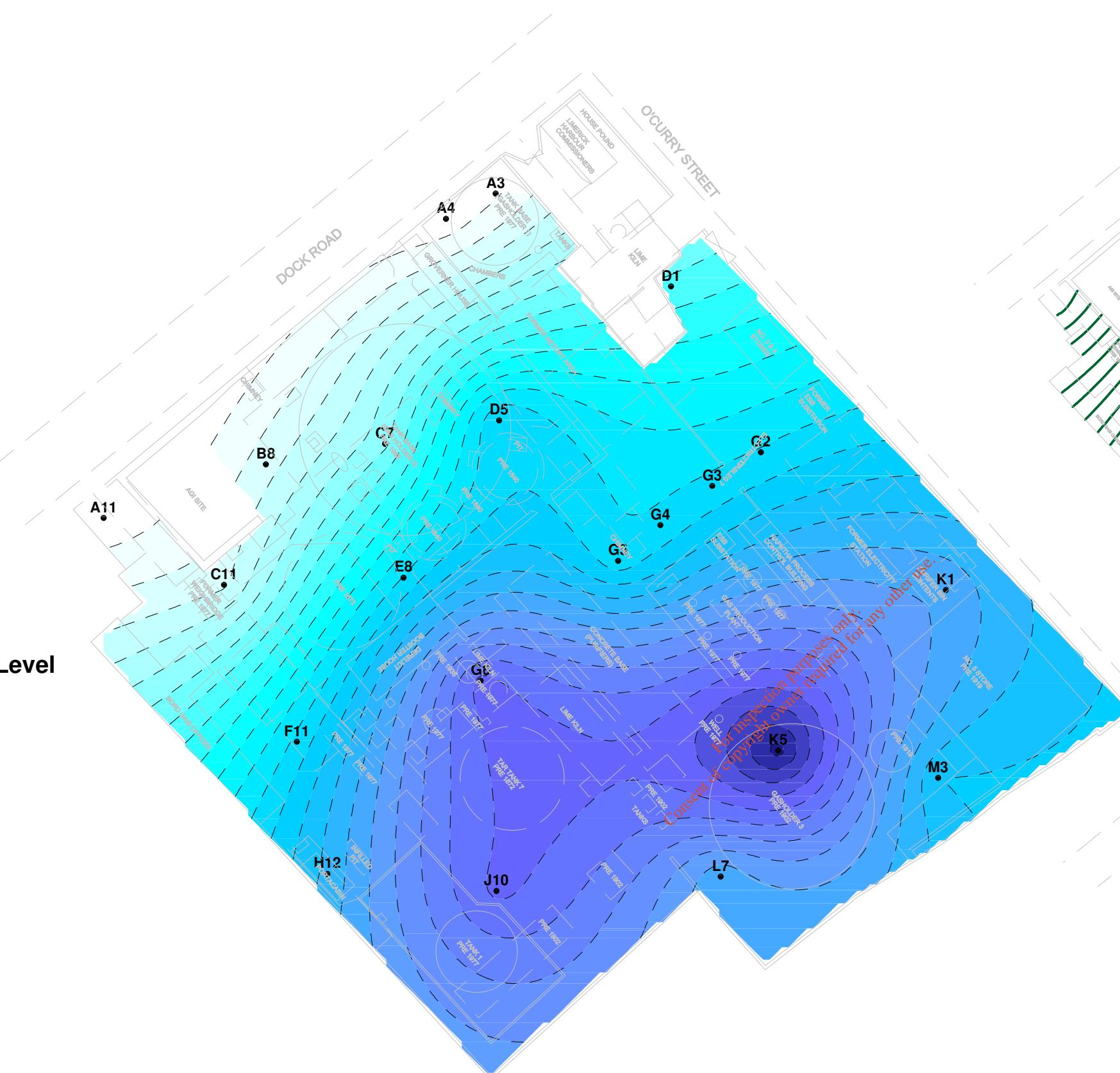
These plots have been produced using data obtained from the groundwater monitoring visit undertaken on 26-27/01/2011. Contours were plotted using the Kriging method based upon a 1m x 1m grid.
