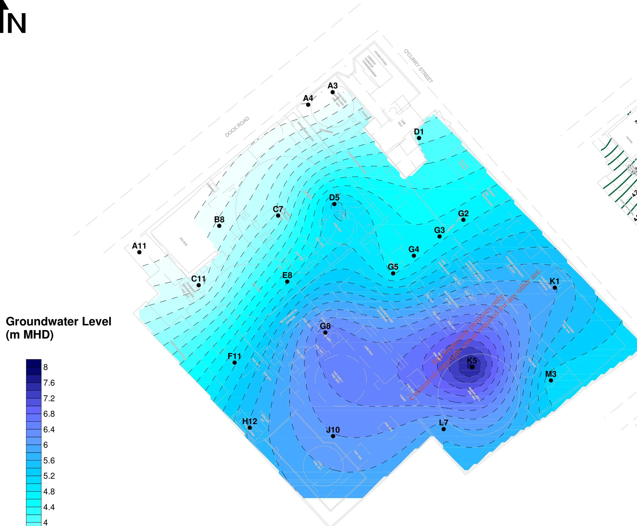
These plots have been produced using data obtained from the groundwater monitoring visit undertaken on 26-27/04/2011. Contours were plotted using the Kriging method based upon a 1m x 1m grid.
