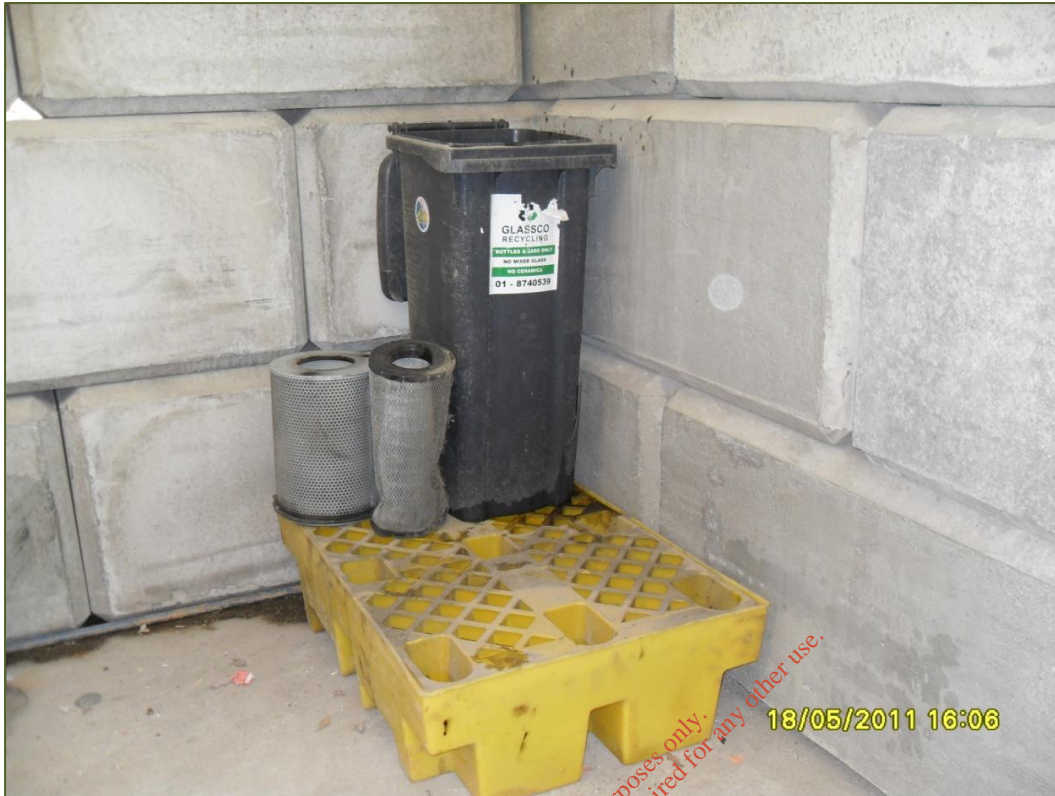
Photograph D.1.13: Spill pallet in garage building
