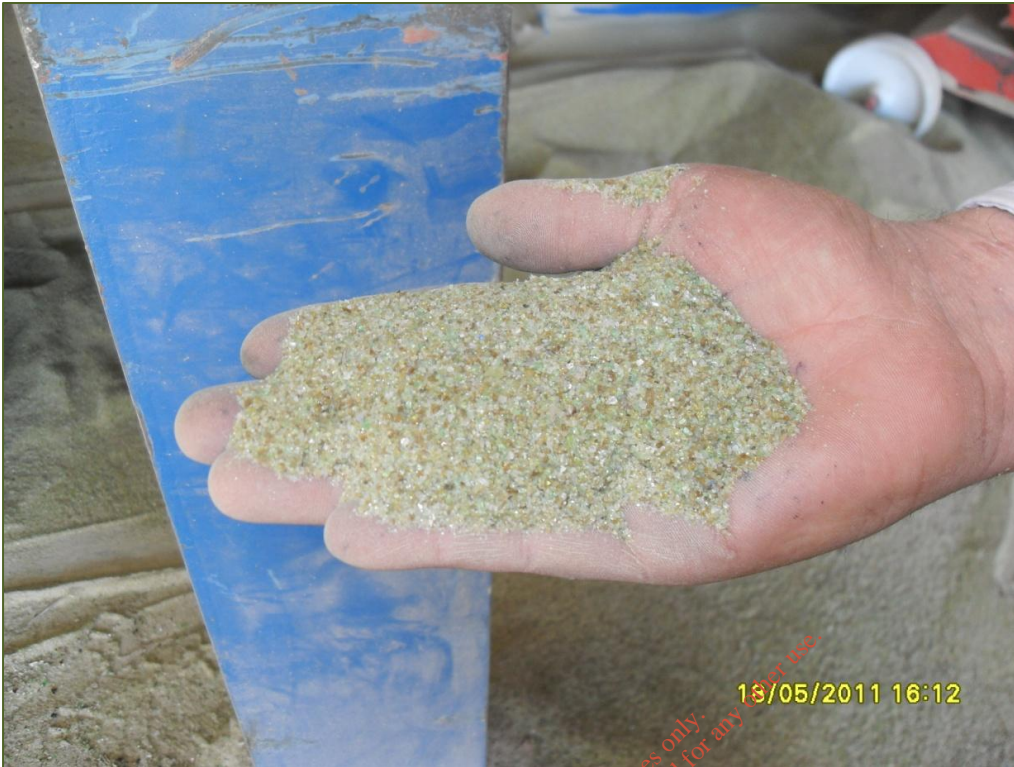
Photograph D.2.9: Crushed and graded product from the Drying Plant
