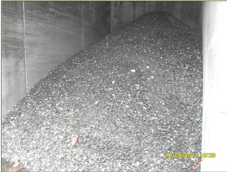
Photograph D.2.3: Clean/separated glass cullet output
