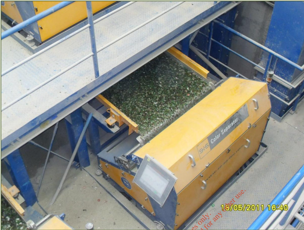
Photograph H.3.2: Spectrum Unit showing glass input conveyor
