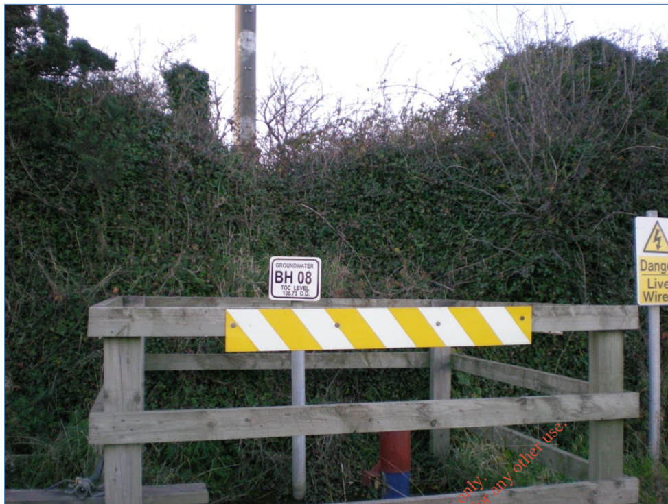
Photograph F.1: Example of existing groundwater monitoring borehole
