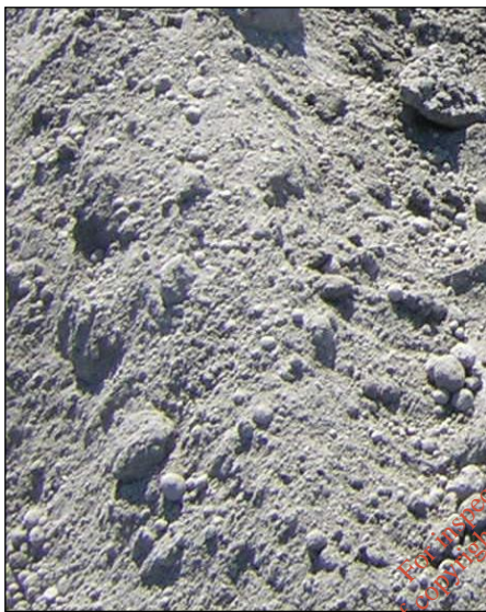
Figure H.1.1: 'Raw' Flue Gas Treatment Residue (from waste-to-energy facility)
