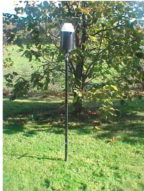
Plate 3.2: Bergerhoff Dust Gauge
