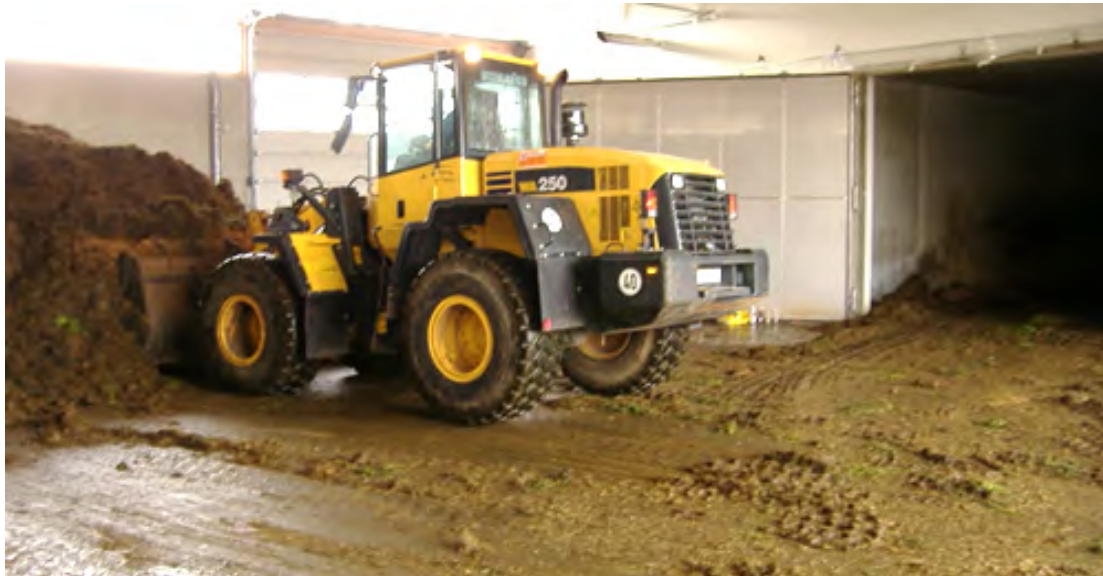
Fig. 7. Filling of a fermentation chamber with Bio-waste.
