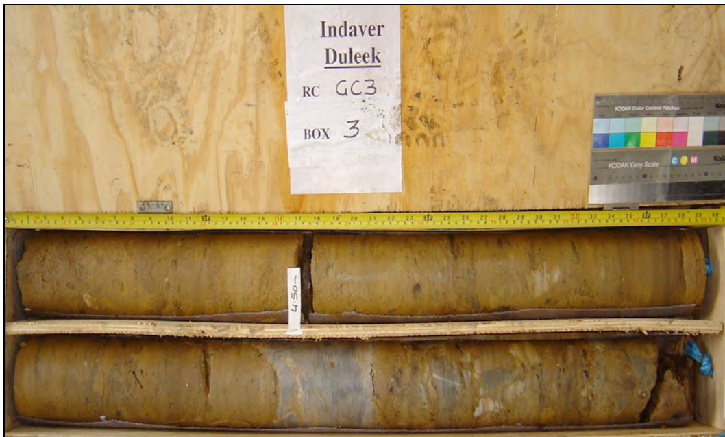
Plate 1 – Geobor Recovery in Glacial Till (GC 3)
